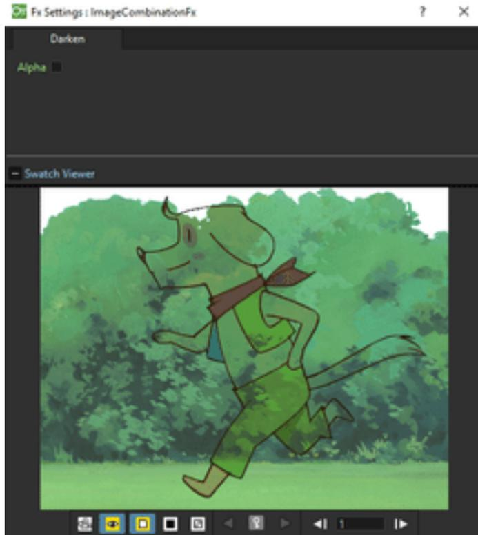
Compares the pixels color of the Up and Down node content and selects the darker one as the result color. The white in the Up node content does not affect the result; the black gives a black result.
