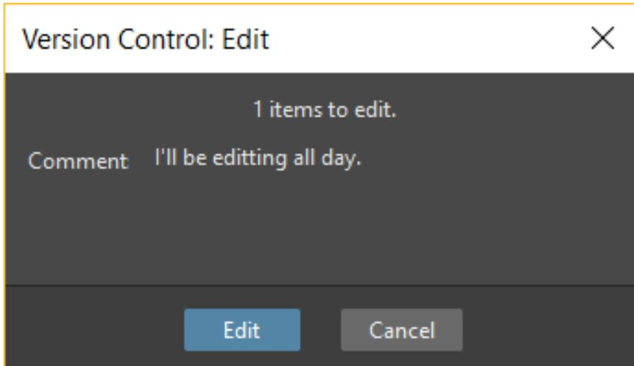
The **Edit** operation “locks” the file, so only the user running the command will be able to modify it (preventing other users using the same *central repository* from unlocking it and being able to modify it). At the moment a file is about to be edited, it’s possible to type in a *Comment*, to let the other users know about your editing operation.
