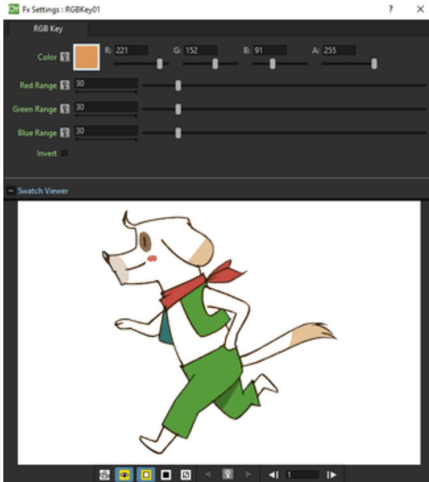
Defines a chroma key for the Source content using the set Red, Green and Blue values. You can set the range for each value by using the related Range slider. The selection can be inverted using the Invert button.
