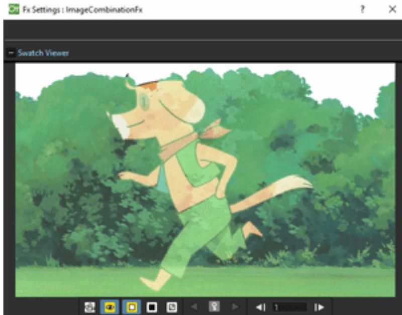
Combines by multiplying the inverse of the pixels color of the Up and Down node content, giving a result color that is lighter than both Up and Down node pixels, except when one of them equals 0. The black in the Up node content does not affect the result; the white gives a white result.
