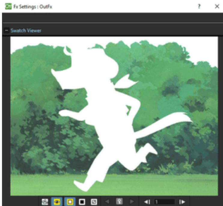
Makes the source content visible only outside the opaque areas of the node content connected to the Matte input port.
