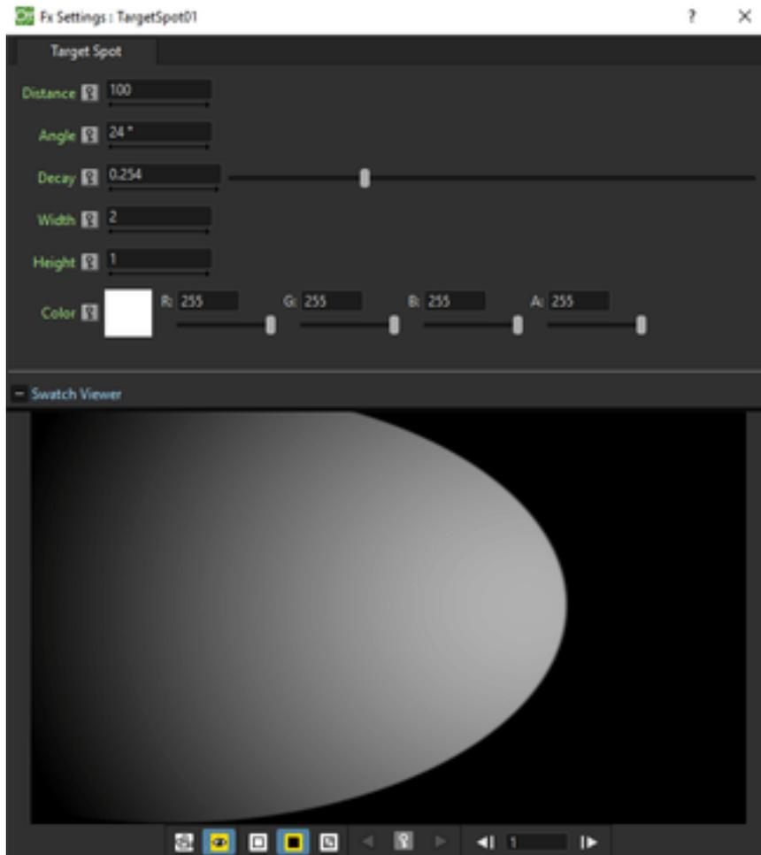
Creates a new column/layer containing a light spot whose size and color can be set respectively with the Width and Height values, and the Red, Green, Blue and Alpha values. The direction of the spot can be set by defining the Distance of the light from the table and the Angle between the light spot direction and the table. The Decay, that is the decrease of the light intensity according to the distance from table, can be controlled as well.
