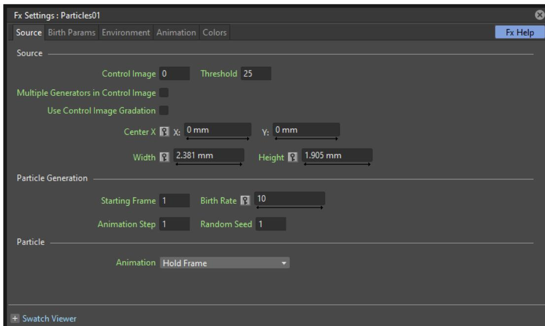
The particles Source is the area where the particles are generated. It can be defined in the **Source** page, by specifying its size and position, or a control image. The way particles are generated, for example their birth rate, can be controlled as well.
