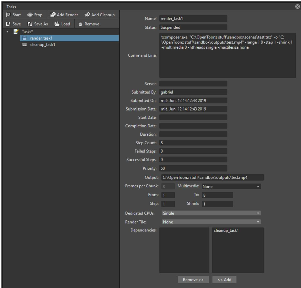
The Tasks pane is divided into two sections: on the left there is the Task tree where all of the *Render tasks* are displayed with a clapboard icon and all the *Cleanup tasks* with a brush icon; on the right there is Information about the task selected in the Task tree.
