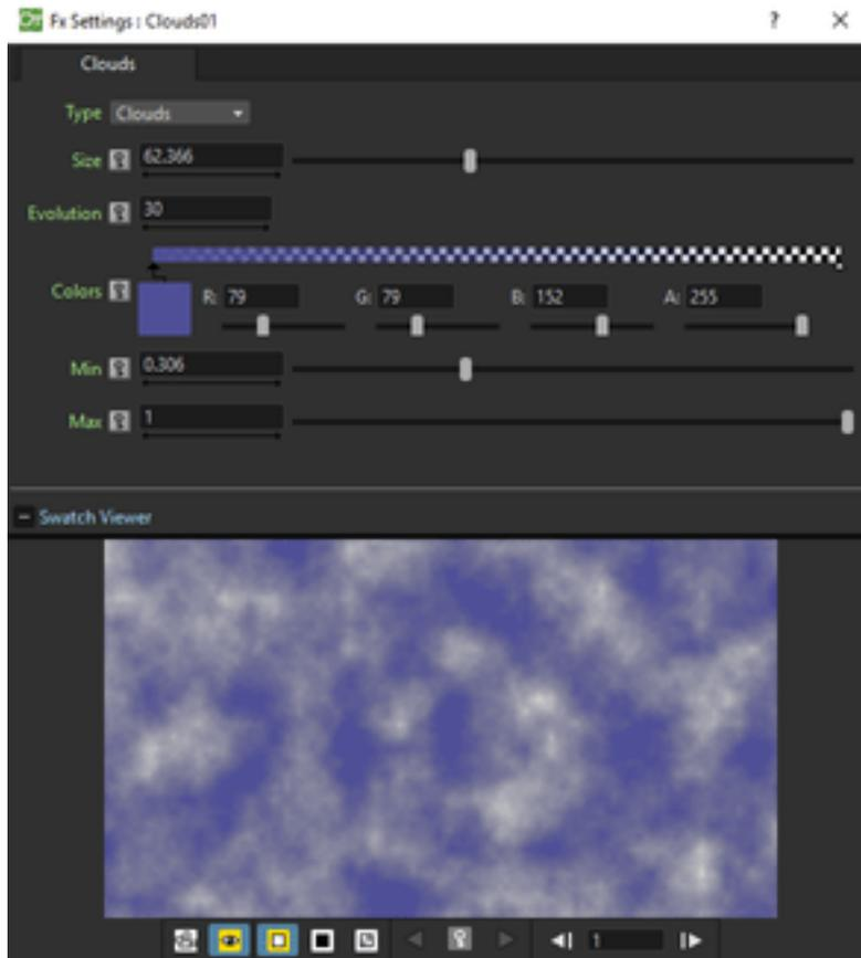
Creates a new column/layer containing a fractal image whose type can be chosen between Clouds and Marble/Wood. The Size affect the grid used for generating the fractal image; a color spectrum defines the used colors (see [Defining Colors and Color Spectrums](#) ).
