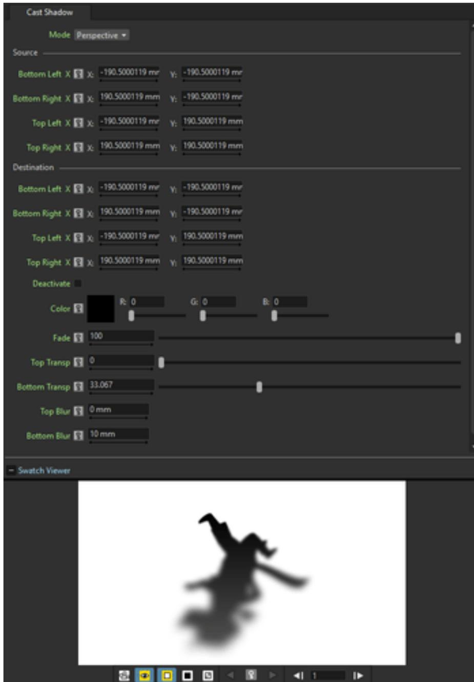
Turns the Source content into a shadow that can be distorted and faded to a color with a variable transparency and blur. The distortion can be done like in the Free Distort effect (see *Free Distort* ). The fade Color can be defined by Red, Green and Blue values and a Fade intensity can be set. A different Blur and Transparency value can be set for the top and the bottom part of the Source content, in order to have a more realistic shadow.
