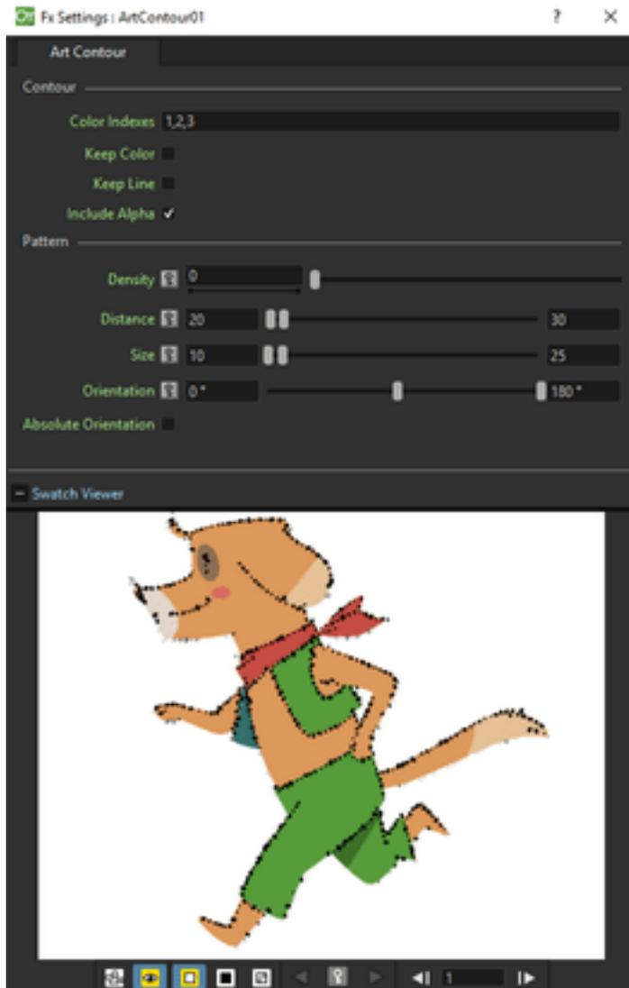
Creates in the Source content a pattern, by repeating the Controller node content, along lines painted with styles whose indexes are specified in the Color Indexes text field. It can be used for example to create scattered brush, or hair and fur effects along drawing lines.
