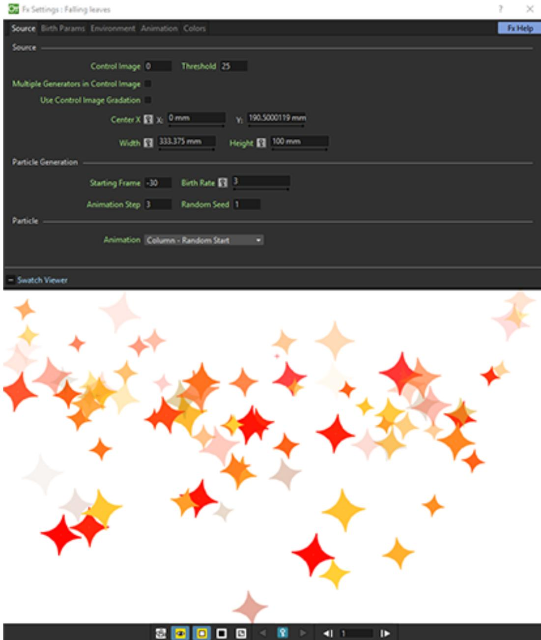
The Particles effect creates a new level in the selected column/layer containing particles.
