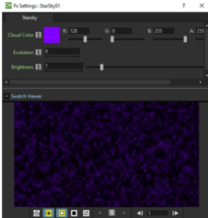
Creates a new column/layer containing a simple star field with variable brightness with overlaid clouds. Sets the color of the overlaid clouds defining the RGBA values of the Cloud Color parameter.
