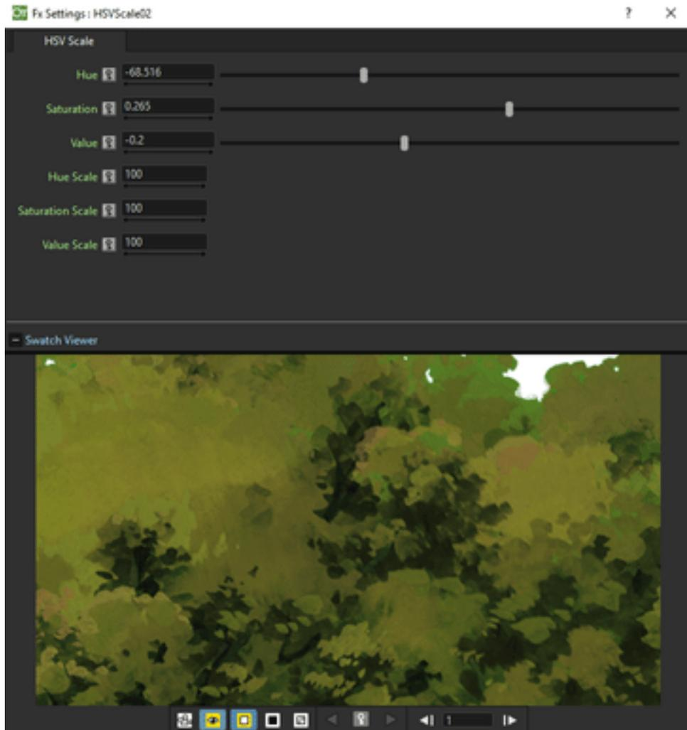
Shifts the Hue, Saturation and Value values of the Source content. Hue ranges from -180 to 180; Saturation and Value from -100 to 100. All the three settings preserve their original value at 0.
