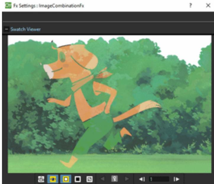
Compares the pixels color of the Up and Down node content and selects the lighter one as the result color. The black in the Up node content does not affect the result; the white gives a white result.
