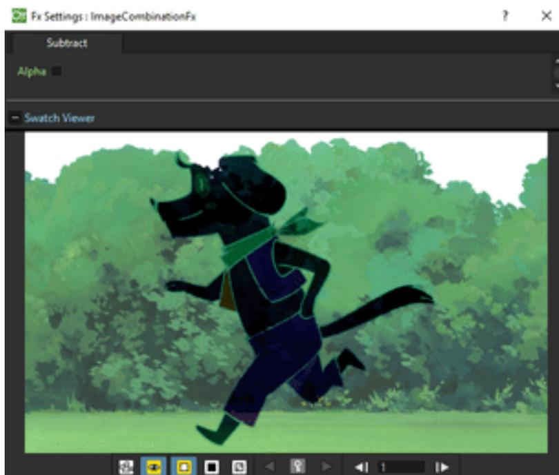
Subtracts the red, green and blue values of the Up node content from the Down one, pixel by pixel. By activating the Alpha option, also the alpha information is considered.
